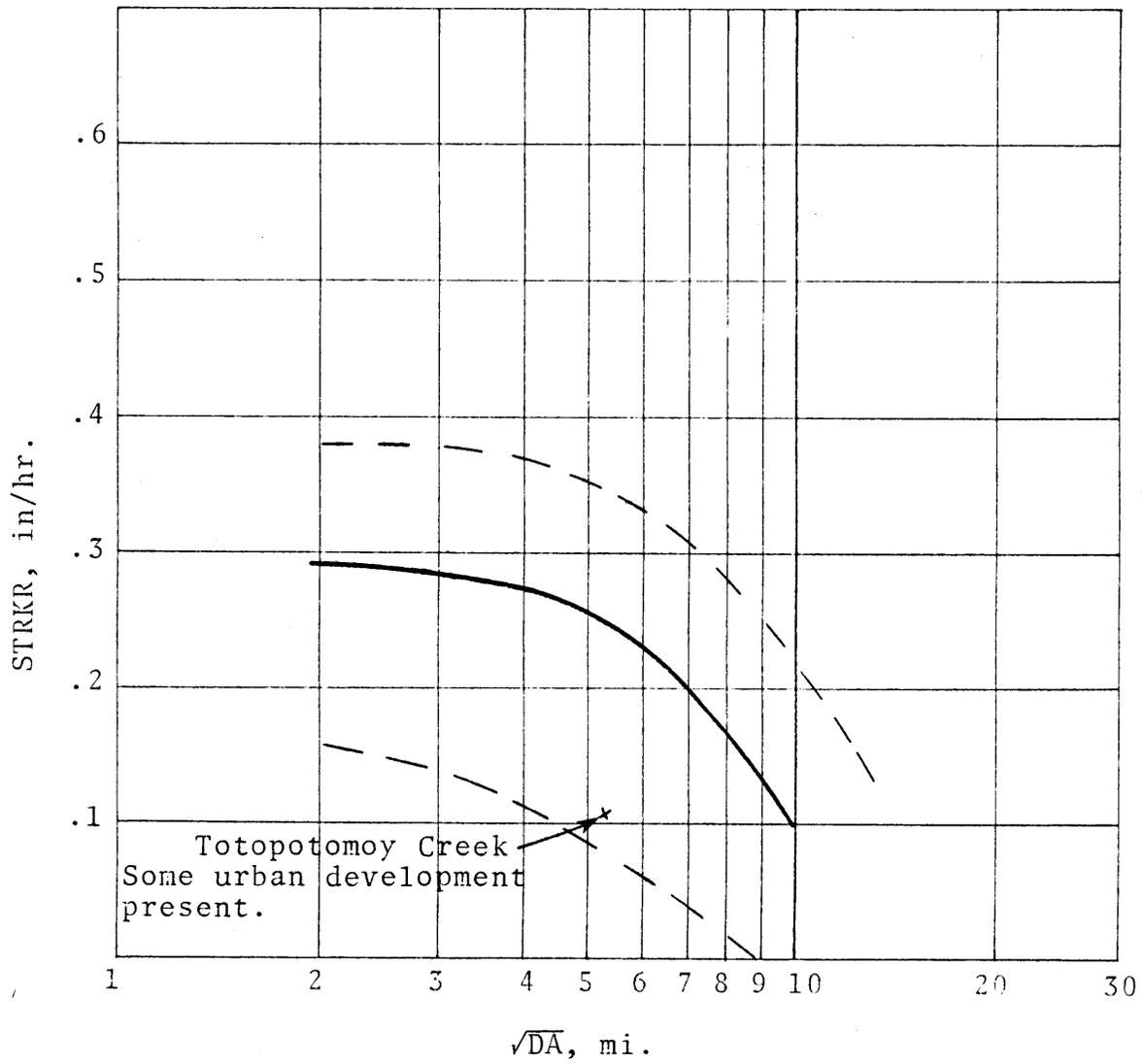
Figure A-23. Parameter selection curve, STRKR for Region C1378-C25.
