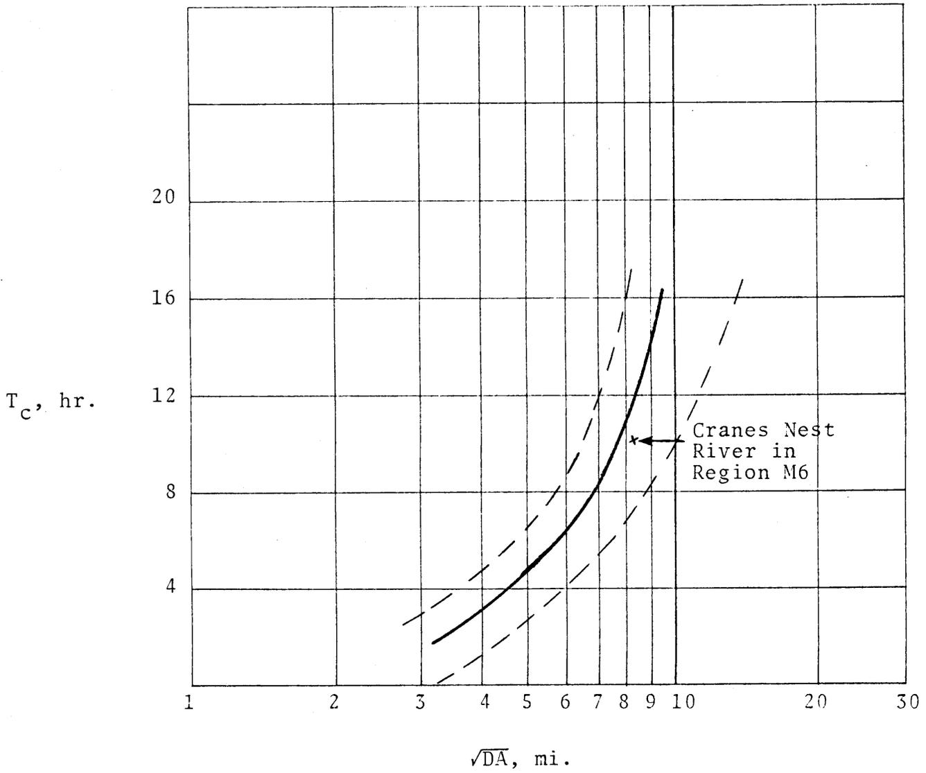
Figure A-25. Parameter selection curve,  $T_c$  for Region M649-M6.
