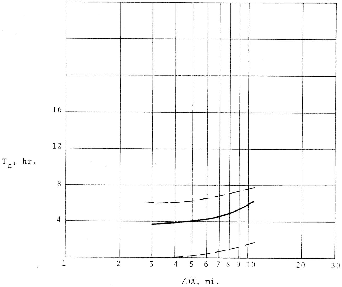
Figure A-17. Parameter selection curve,  $T_c$  for Region M2-M1.
