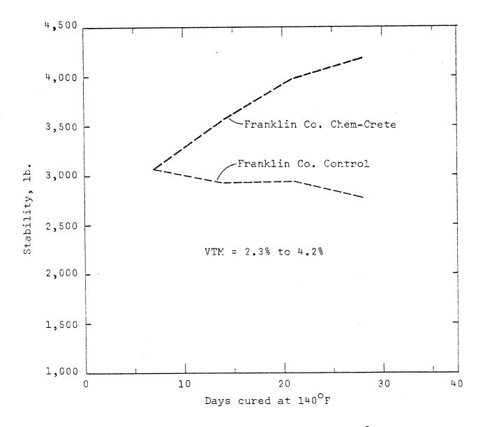
Figure 4. Marshall stability vs. days at 140°F for specimens compacted with 50 blows. Tests by Materials Division. 1 1b. = 4.45 N; °C = 9/5 (°F-32).
