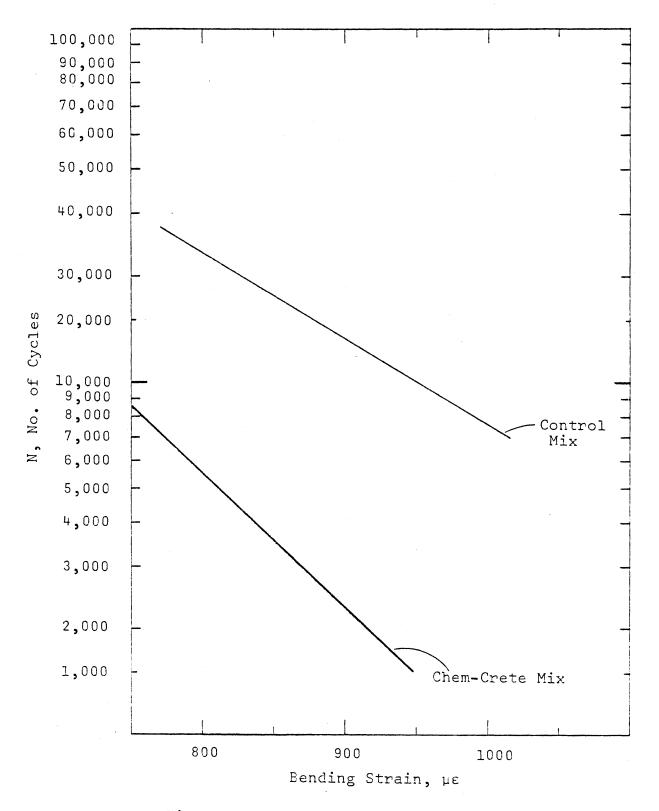
Figure 7. Constant strain fatigue tests.
