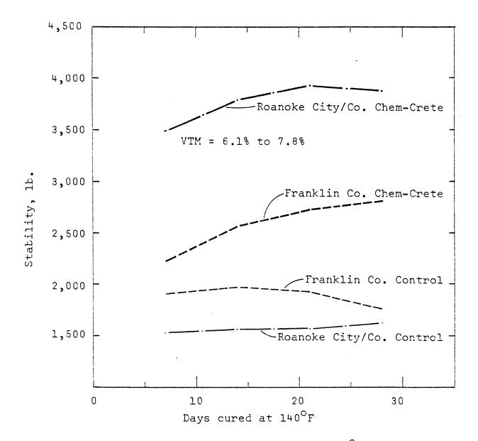
Figure 3. Marshall stability vs. days at 140°F for specimens at pavement density. Tests by Materials Lab. 1 lb. = 4.45 N; °C = 9/5 (°F-32).
