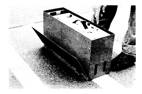
Figure 14. Retroreflectance meter.
