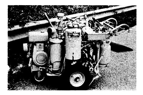
Figure 1. Paint striping machine.
