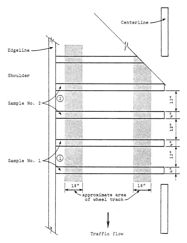
Figure 9. Placement of test materials.
