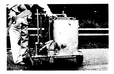
Figure 6. Machine for applying thermoplastic.
