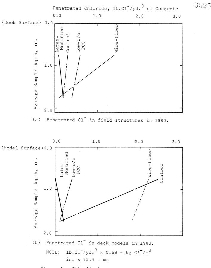
Figure 6. Chloride ion contents measured by titration analysis.
