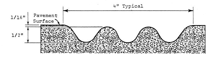
Figure 1. Cross section of groove. Note: 1 inch = 2.54 cm.
