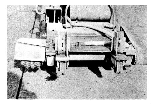
Figure 3. Concrete saw modified to accommodate special diamond drum cutter.
