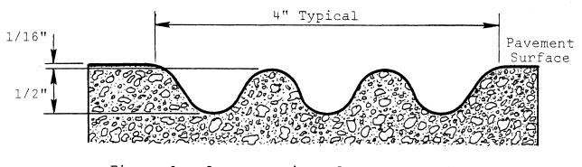
Figure 1. Cross section of groove. Note: 1 inch = 2.54 cm.
