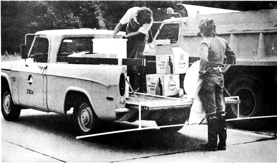
Figure 5. Apparatus for spreading acid.
