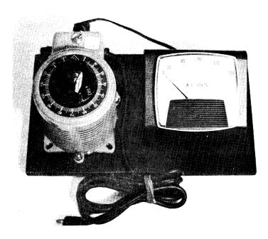
Figure 9. Variable autotransformer and voltmeter.
