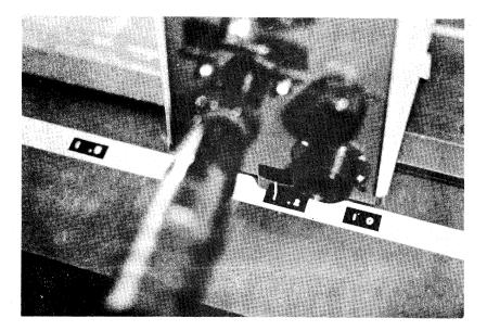
Figure 19. Receiver carrier divergence angle settings.
