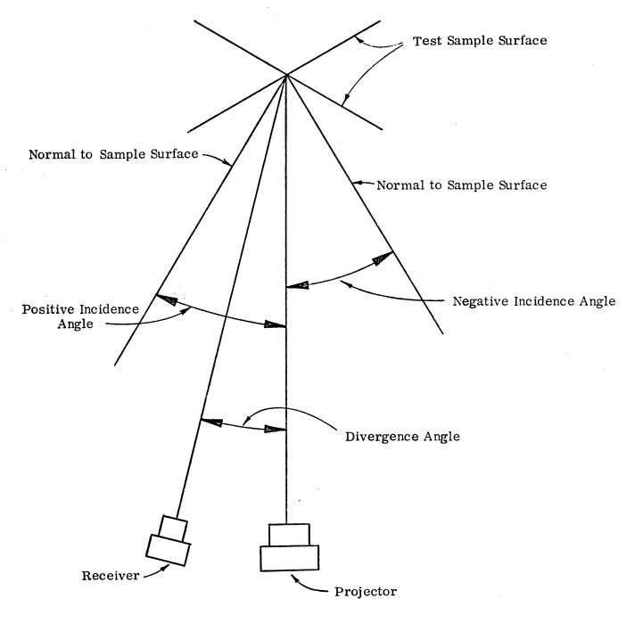
Figure 1. Incidence and divergence angles.
