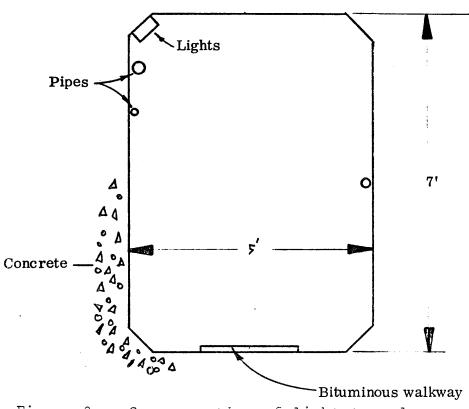
Figure 3. Cross section of light tunnel.
