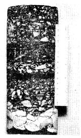
Figure 1. Core showing typical number of overlays on concrete base.
