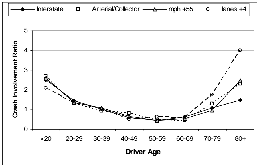
Figure 16. Two-vehicle fatal CIRs for changing lanes or merging on various types of roadways.
