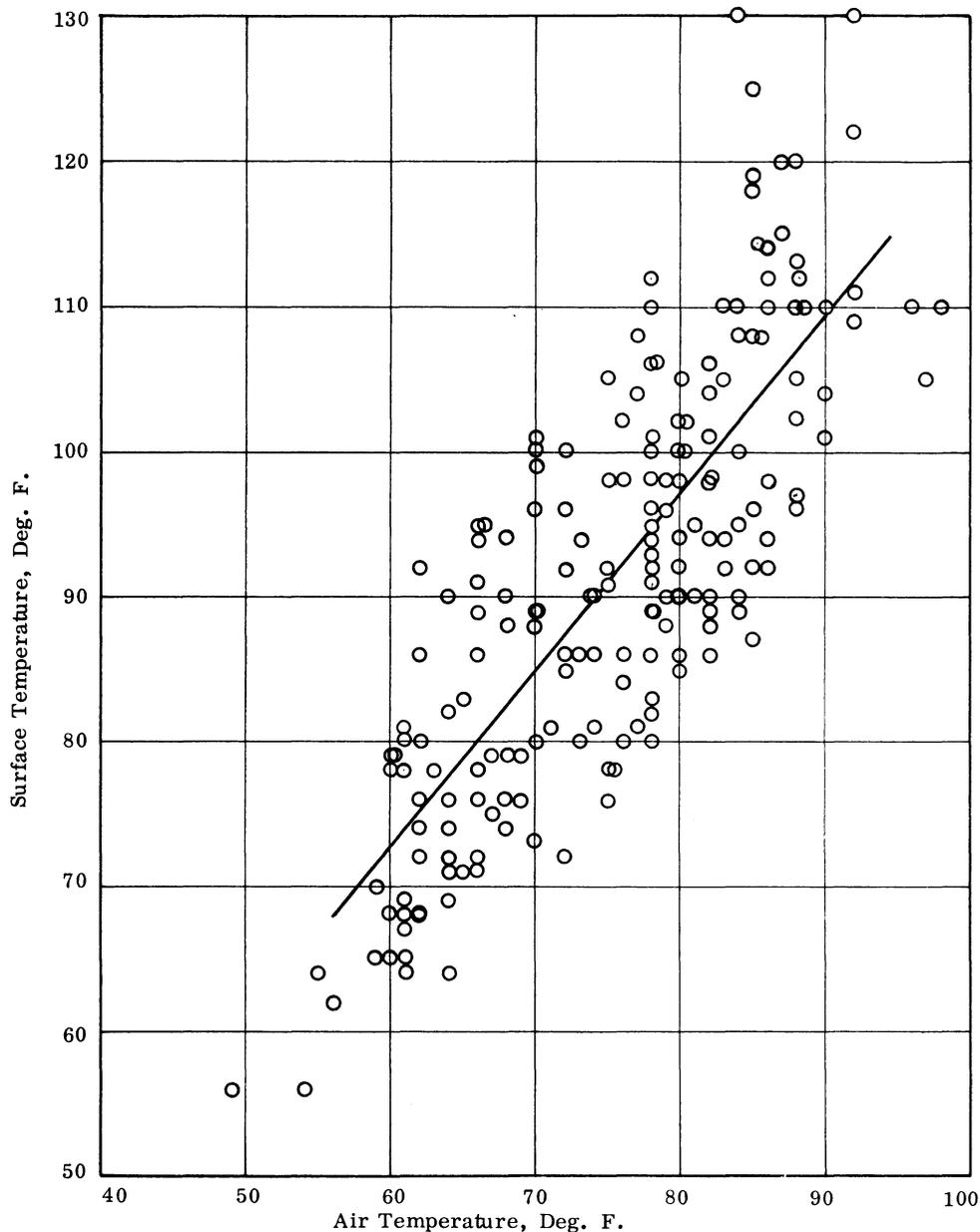
Figure 1. Relationship of air and surface temperature.
