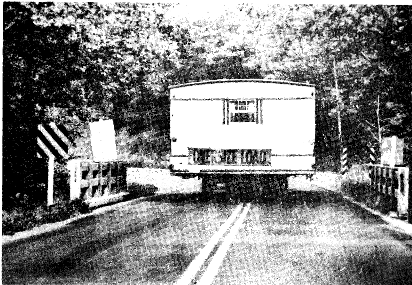
Figure 20. Wide loads frequently encroached into the opposing traffic lane on narrow two-lane highways.
