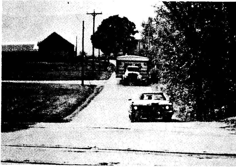
Figure 19. Twelve- and 14-foot housing units continuously encroached into the adjacent lane on secondary facilities.
