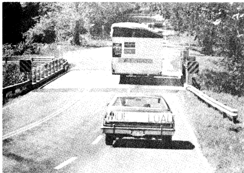
Figure 21. Encroachment at narrow structures.
