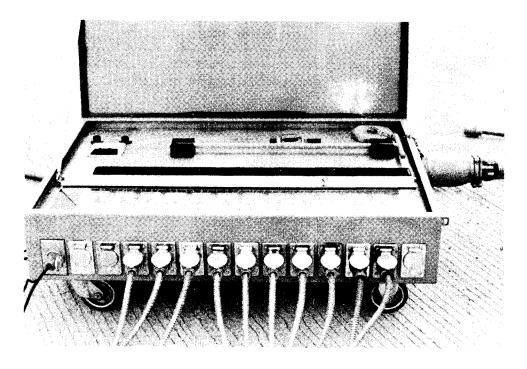
Figure 19. Control panel for electrical distribution to heating blankets.
