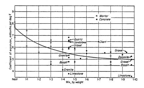
Figure 11. Thermal coefficients of expansion of neat cements, mortars, and concretes.(2)
