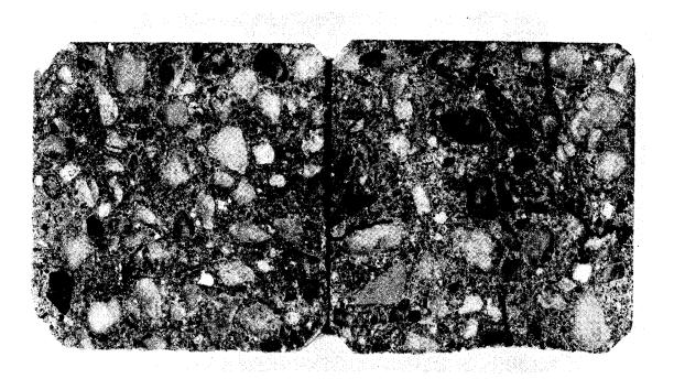
Figure 12. Polished sections from unheated (left) and heated (right) 3 x 3 x 11 in. (76 x 76 x 279 mm) prisms.
