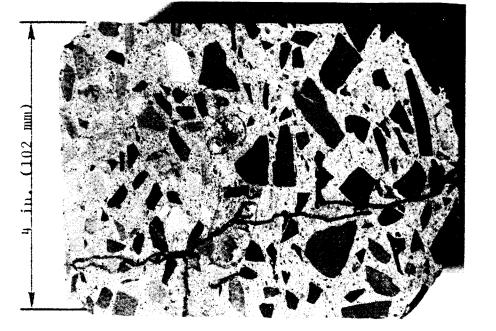
Figure 16. Core through overlay and raked base layer.
