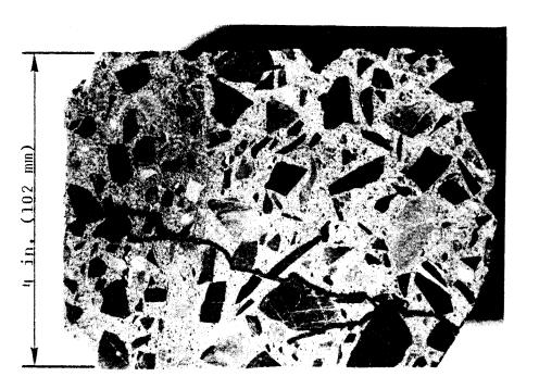
Figure 17. Core through overlay and screeded base layer.
