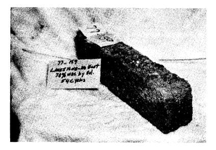
Figure 6. Freeze-thaw specimen with scaling type failure.
