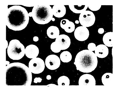
Figure 1. Spherical wax beads with air voids (dark spots). 63x
