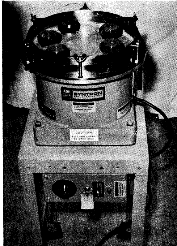
Figure 4. Vibratory polishing lap. Weights with "O" ring bumpers over thin sections.
