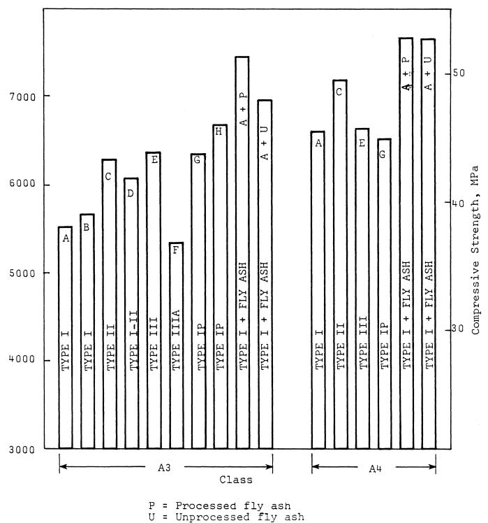
Figure 1. Compressive strength values at 6 months. NOTE: Letters denote the sources which are included in Appendices A-5 and A-6. (NOTE:
