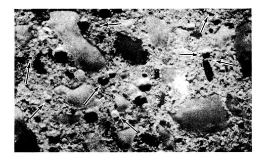
Figure 5. At top, polished surface (24x); bottom, etched surface (45x). Fly ash particles are indicated by arrows; remaining voids are assumed to be air bubbles. 0527
