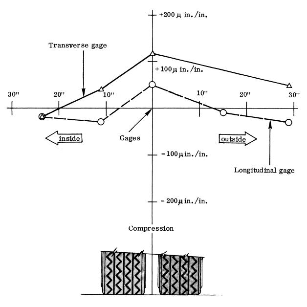
Figure A-1. Influence diagram for surface strain at £ of established wheelpath - Route 20.
