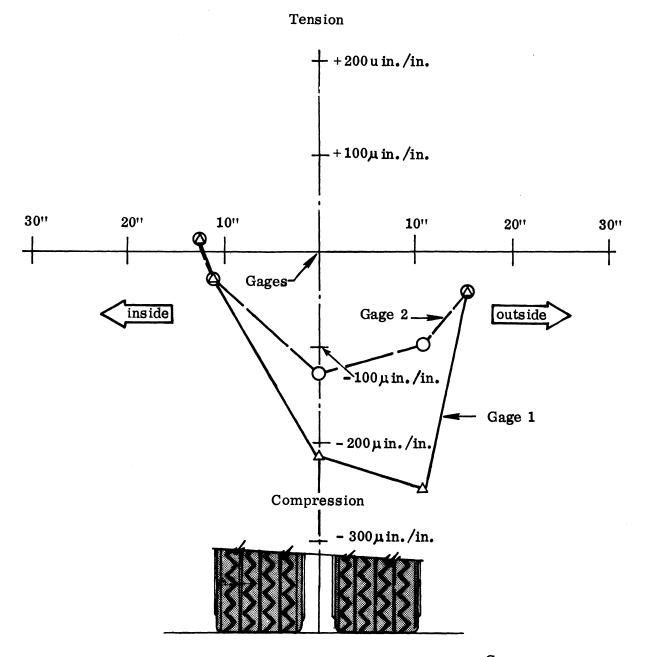
Figure A-2. Influence diagram for surface strain at £ of established wheelpath - Route 250.
