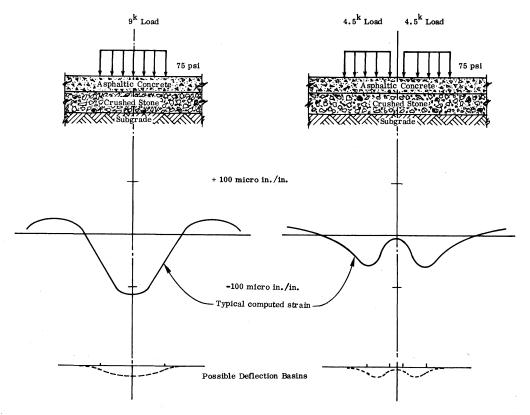
Figure 2. Load configurations used to compute strains.
