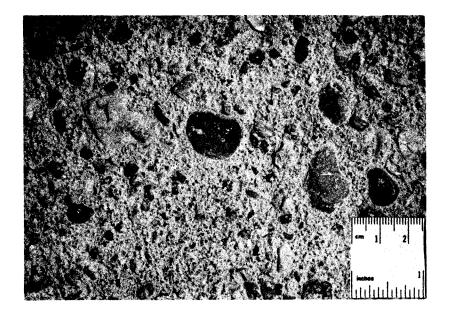
Figure 8. Exposed aggregate texture. Site 3.
