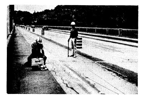
Figure 12. Corrosion potential measurements in progress.
