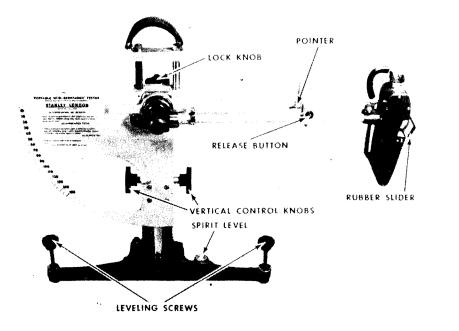
Figure 8. British Portable Skid Resistance Tester.
