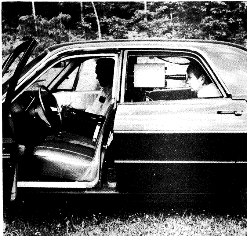
Figure 1. Telephotometer used to measure sign luminances.
