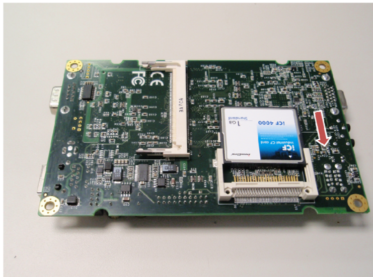
Figure B.51: Insert compact flash card into ALIX board
