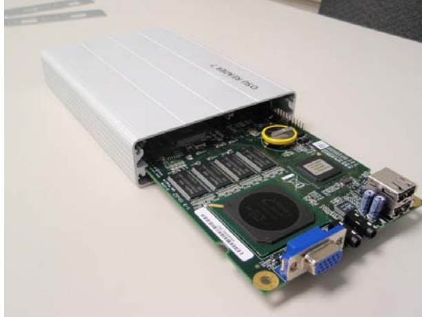
Figure B.52: Slide ALIX board into enclosure
