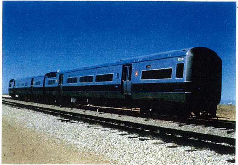
A 1975 photo of the gas turbine/electric train built by Garrett AiResearch for the New York MTA. The MTA used this and a trainset built by GE to compare gas turbines vs. electrification for extending its commuter rail lines.
