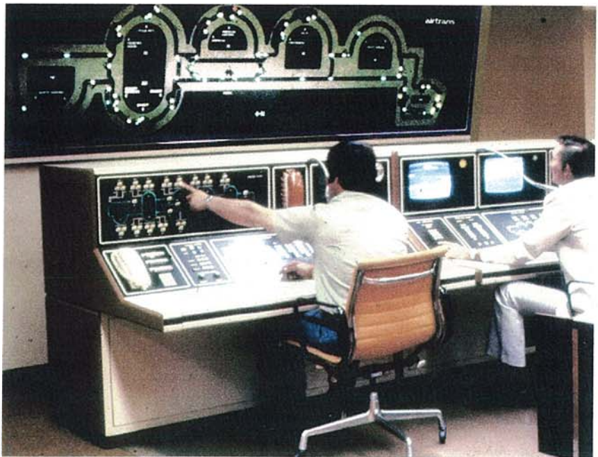
This control center at Dallas/Fort Worth Airport is capable of directing automated vehicles on several different routes to deliver passengers, baggage, mail, and trash.
