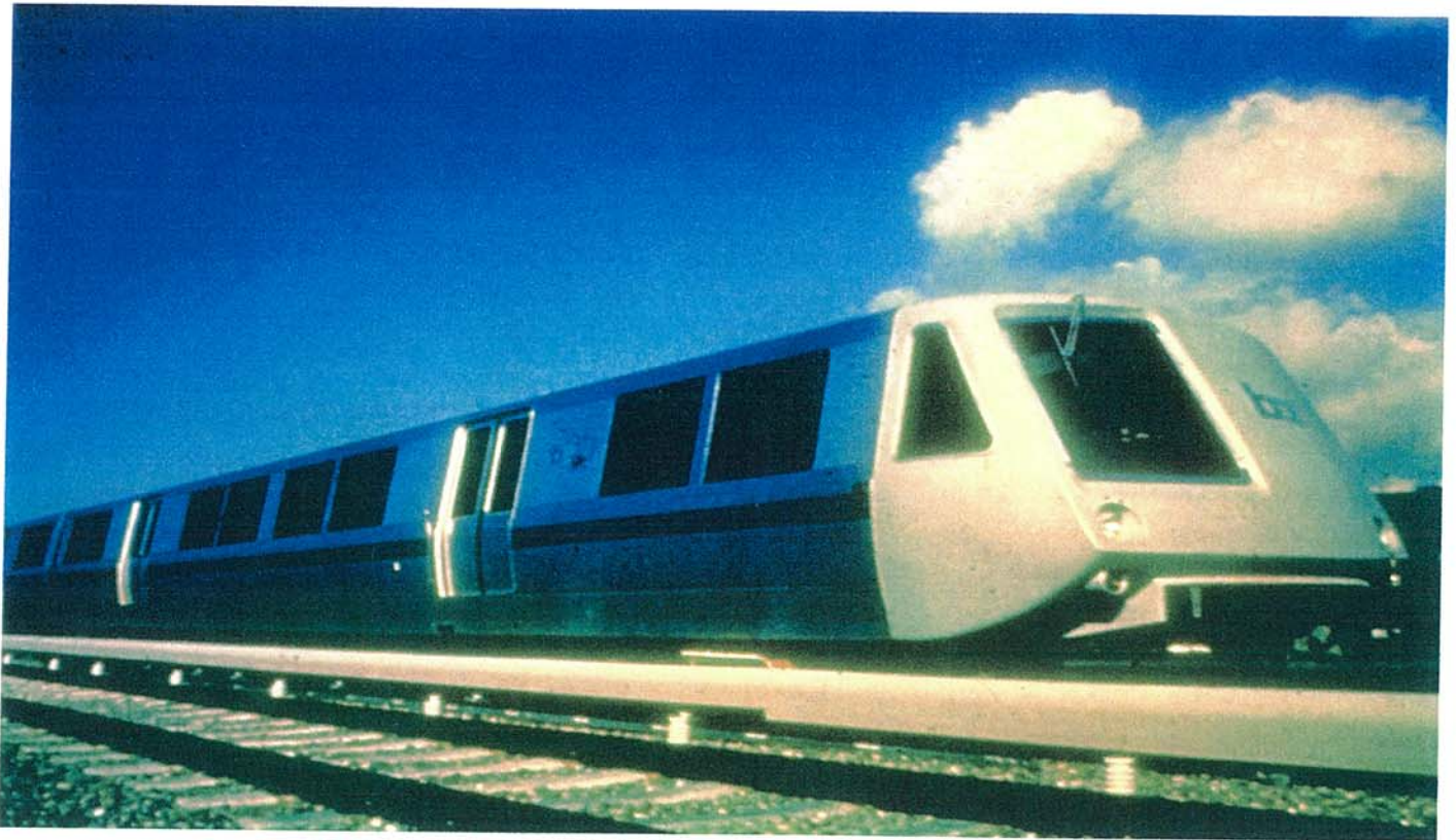
This is a 1971 publicity photo of the BART prototype train which was designed and manufactured by Rohr Corporation of Chula Vista, California. Cars had aluminum bodies, were air conditioned and could operate at speeds up to 80 mph..
