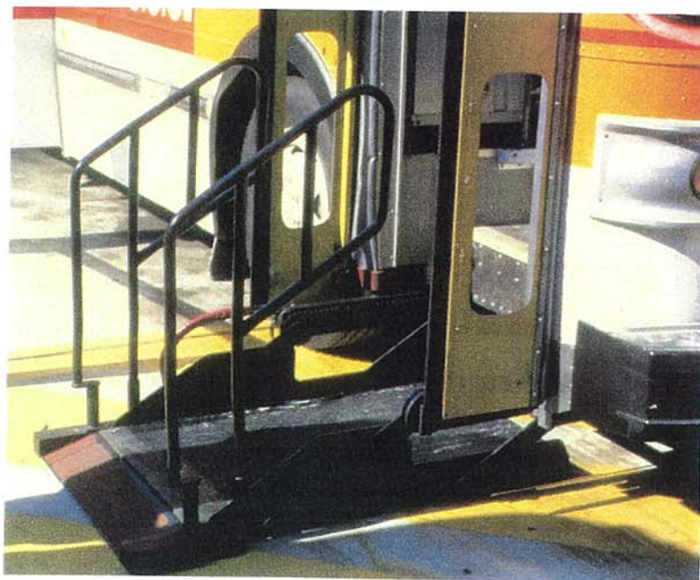
A variety of wheelchair lifts were tested in the 1980's. This front door "steplift" was preferred because the driver could assist riders most efficiently. However, to retain the steps for ambulatory riders, lift mechanisms were complicated.
