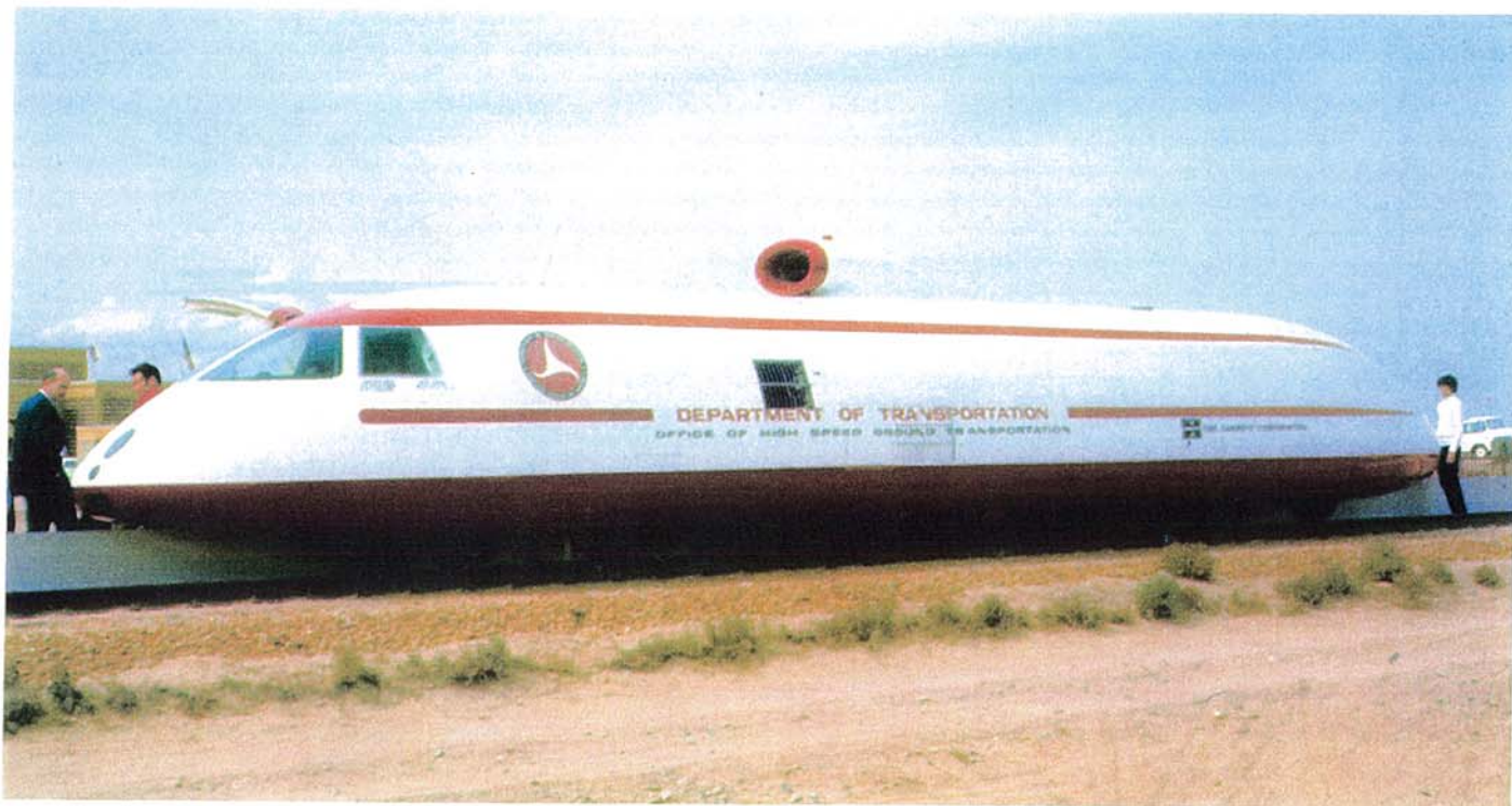
LIMRV - The Linear Induction Motor Research Vehicle (above and below) is shown at the Transportation Test Center in 1972. It was used by the FRA to refine propulsion methods. The aluminum reaction rail is in the center of the tracks. Electrical power was obtained from a turbine powered generator.
