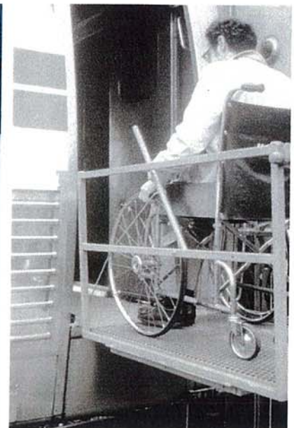
The wheelchair lifts (above) were developed in the late 1970's for light rail and commuter rail systems that required steps for boarding.
