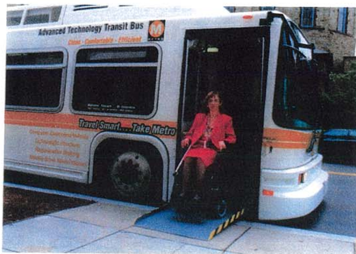
A low floor allows use of a ramp, rather than the more expensive and less reliable lifts.
