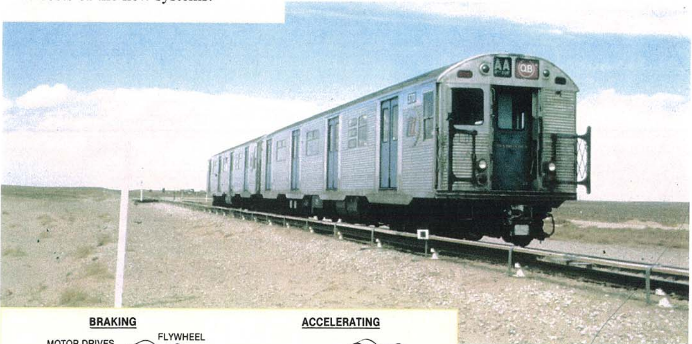
A 1975 photo of the gas turbine/electric train built by Garrett AiResearch for the New York MTA. The MTA used this and a trainset built by GE to compare gas turbines vs. electrification for extending its commuter rail lines.
