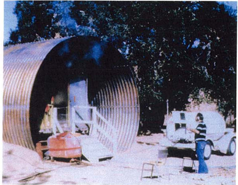
Following a fire in the BART Trans-bay tunnel, UMTA intensified fire safety research. Pictured above are tests of the interior effects of an underbody car fire. Propane burners were used to provide heat in a simulated tunnel (below)..
