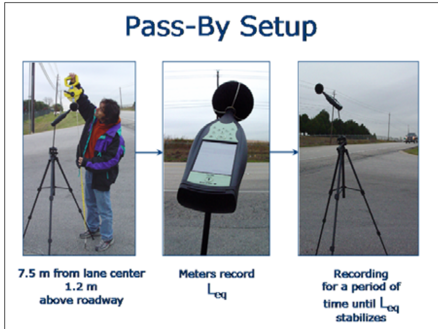
Figure 2.1: Pass-by noise measurements at roadside
