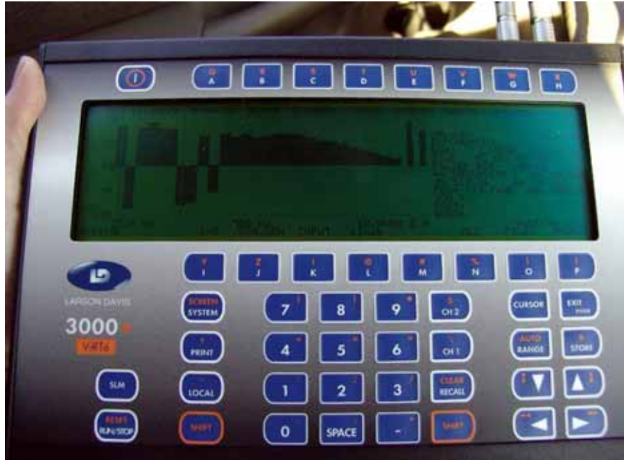
Figure 2.10: Larson Davis 3000+ sound intensity analyzer
