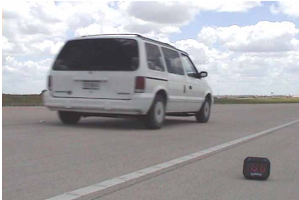
Figure 6.22: Speed recording for pass-by test on SH 130
