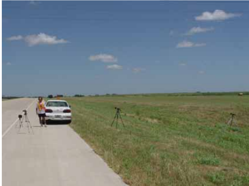
Figure 6.21: Equipment set-up for pass-by tests on SH 130
