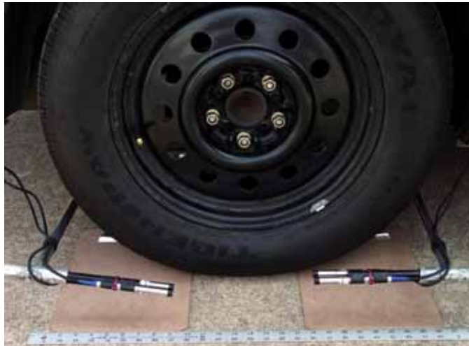
Figure 3.12: Transtec OBSI fixture
