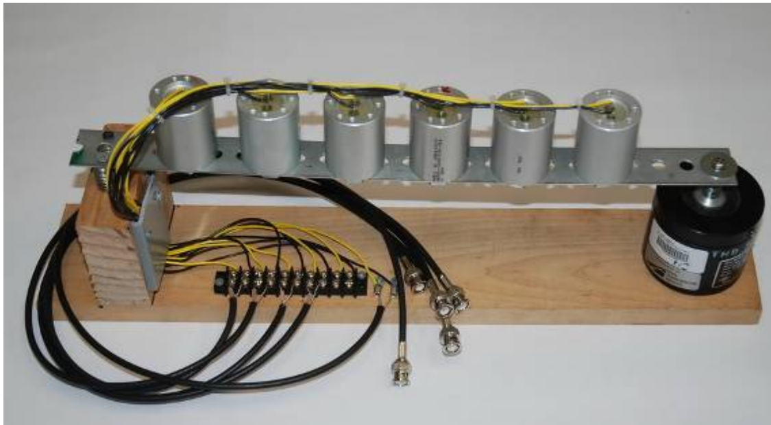
Figure 6.14: TPAD Geophones Simulator Device (Home Made)
