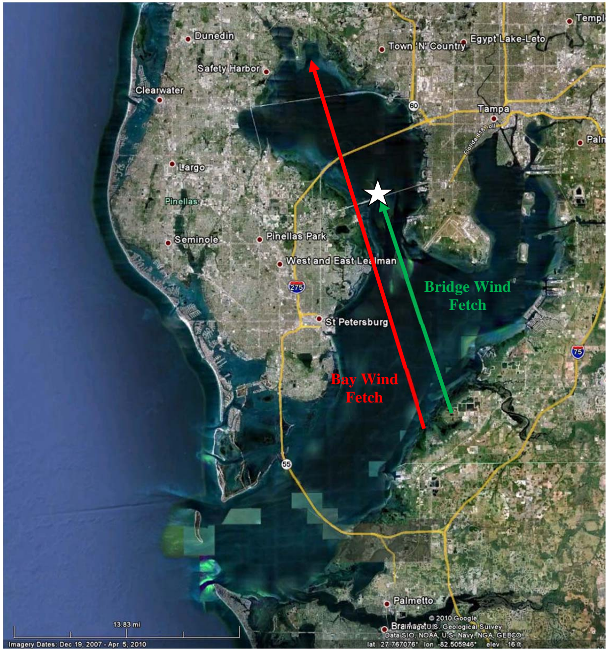
Figure 2-5 Bay wind setup fetch and bridge wind setup fetch for a bridge (shown with the white star) on Old Tampa Bay.
