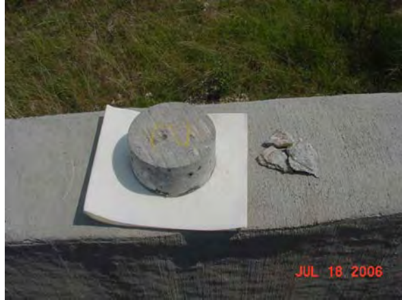
Figure 9: Core #2 – gas bubble hole in center.
