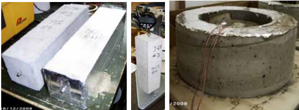
Figure 4-2. Unsealed, sealed, and restrained shrinkage specimens.
