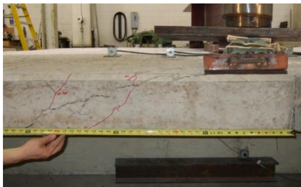
(a) Specimen 1 precast, prestressed overhang
