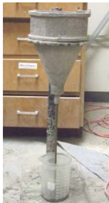
Figure 4-1. Efflux Cone Test.
