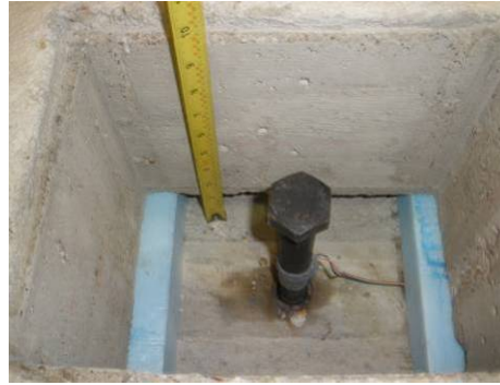
Figure 3-6. Photograph of BC Pre-Installed Shear Connections Specimens.
