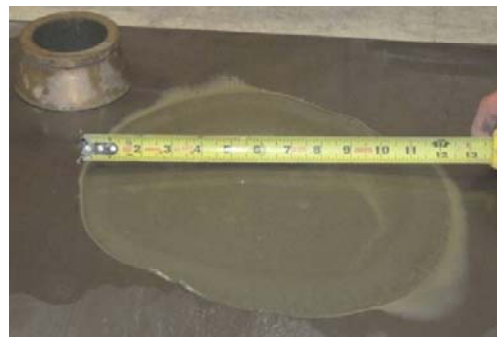
(b) Flow cone showing signs of segregation
