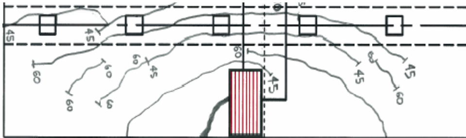
(b) Surface cracks on prestressed-precast overhang. Load increments in kips. Failure load 68 kips (302 kN)
