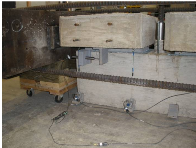
Figure 3-10. Photograph of LVDTs and String Potentiometers Connected to a Shear Test Specimen.
