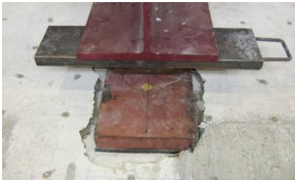
Midpoint (off-set to seam) axle load
