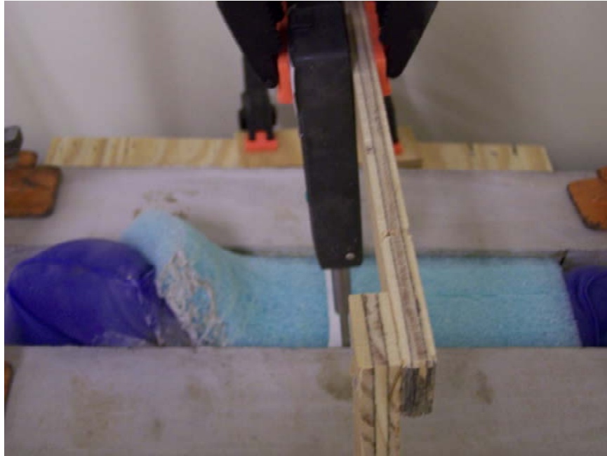
Figure 4-20. A Lateral Pressure Test Specimen at Failure.
