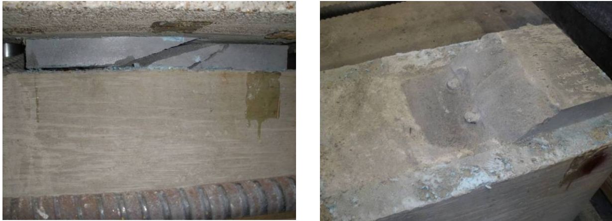
Figure 3-29. 2_NS_2.0 Exhibited a Sliding Shear Failure that Resulted in both NSs Shearing.
