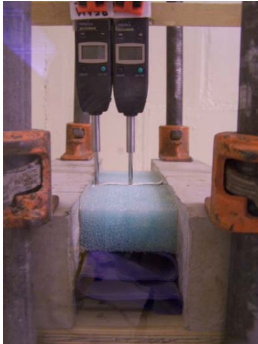
Figure 4-19. Experimental Setup for the Lateral Pressure Test.
