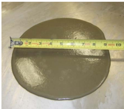
(a) Flow cone displaying good consistency
