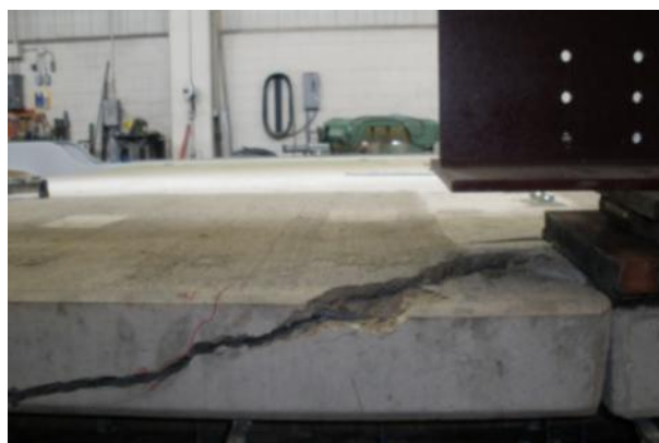
(c) Specimen 2 overhang trailing wheel load
