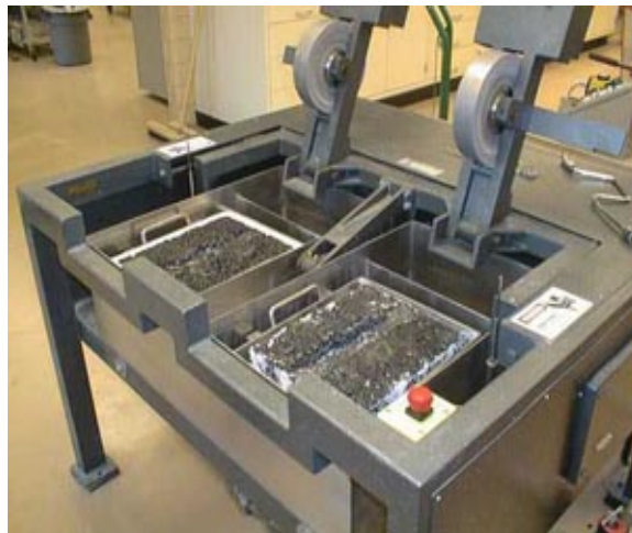
Figure 1.1 Hamburg Wheel Tracking Device (courtesy of FHWA)
