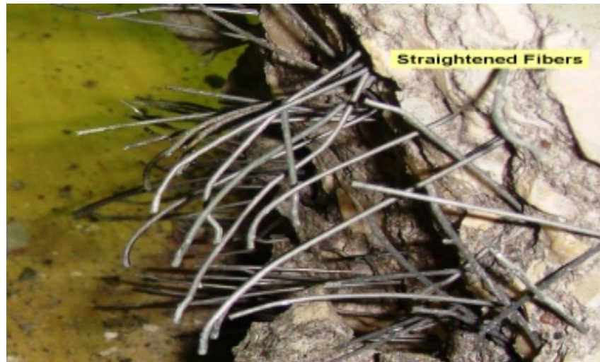
Fig. 3.9 Straightening (De-bonding) of Steel Fibers in Beam Specimen after Failure
