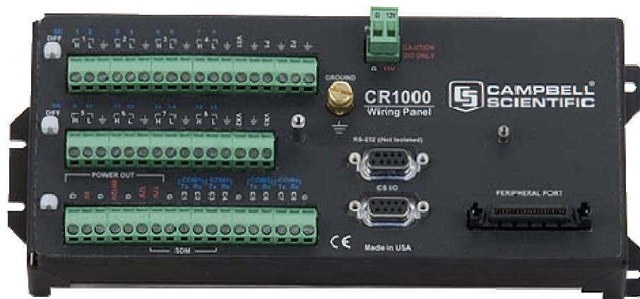
Figure 3-11. CR1000 Datalogger from Campbell Scientific Inc.
