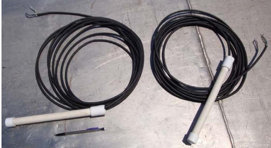
Figure 3-7. TBS Used on US59 over Guadalupe River Bridge.
