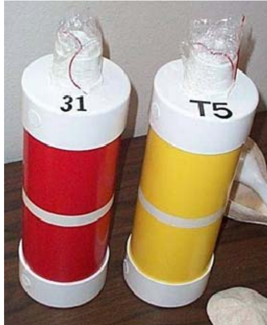
Figure C-6. Float-Out Devices Color Coded and Numbered for Identification (ETI Instrument Systems).
