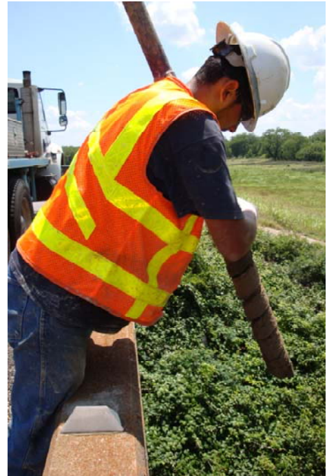
Figure 5-20. Remove Soil from the Drill Bit.
