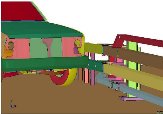
Figure 3.9 Model and physical setup of the New York transition to tubular bridge rail (15)
