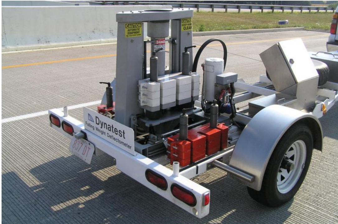
Figure 5.3. ODOT falling weight deflectometer (FWD) used for approach testing
