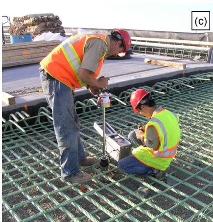
c. Zorn light weight deflectometer (LWD)
