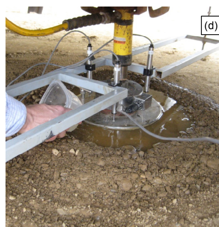
d. Static plate load test (PLT)
