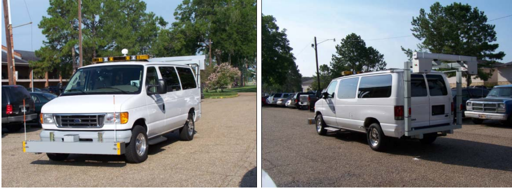
Figure 4 LTRC multi-functional digital highway data vehicle
