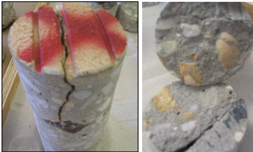
Figure 3-7: Cores from the US 331 deck with vertical and horizontal cracks
