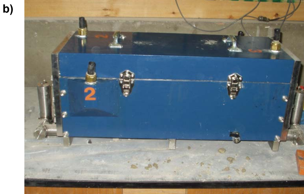
Figure 4-2: Free shrinkage frame test setup: a) Schematic of test (Meadows 2007) b) Actual equipment used
