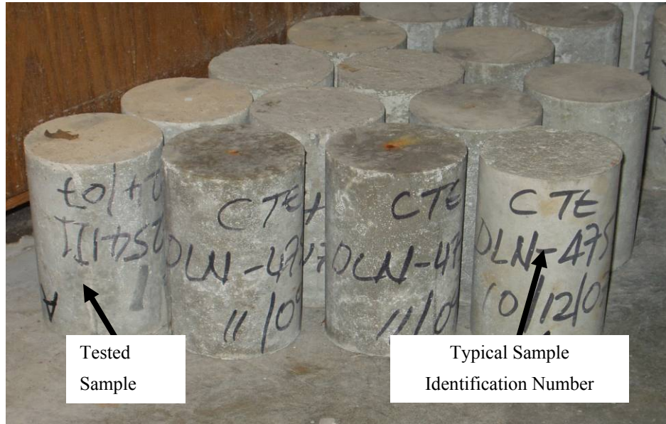
Figure 5-12: Typical tested samples ready to be discarded
