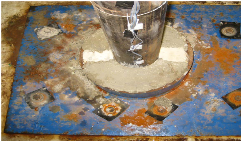
Figure 3-25. Pile to collar connection which is bolted to the bottom plate of laminar soil box
