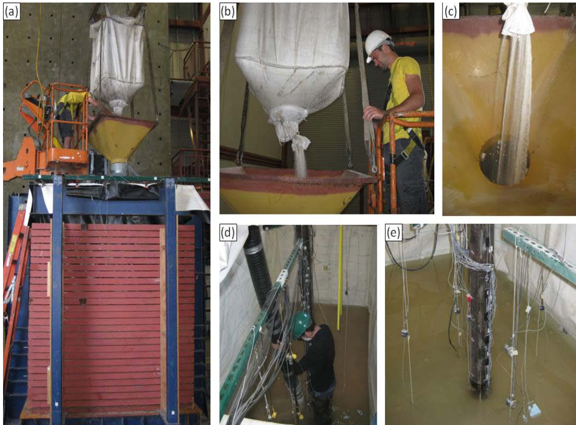
Figure 2-13: (a) Setup; (b) Sand deployment from bag; (c) Sand falling into hopper; (d) Placement of sand in box; and (e) Lift of sand underneath standing water.
