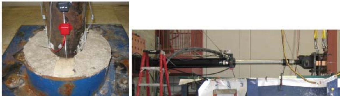
(a) Base of pile to collar connection.
