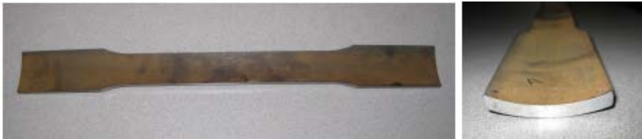
(a) Plan view of test coupon.
