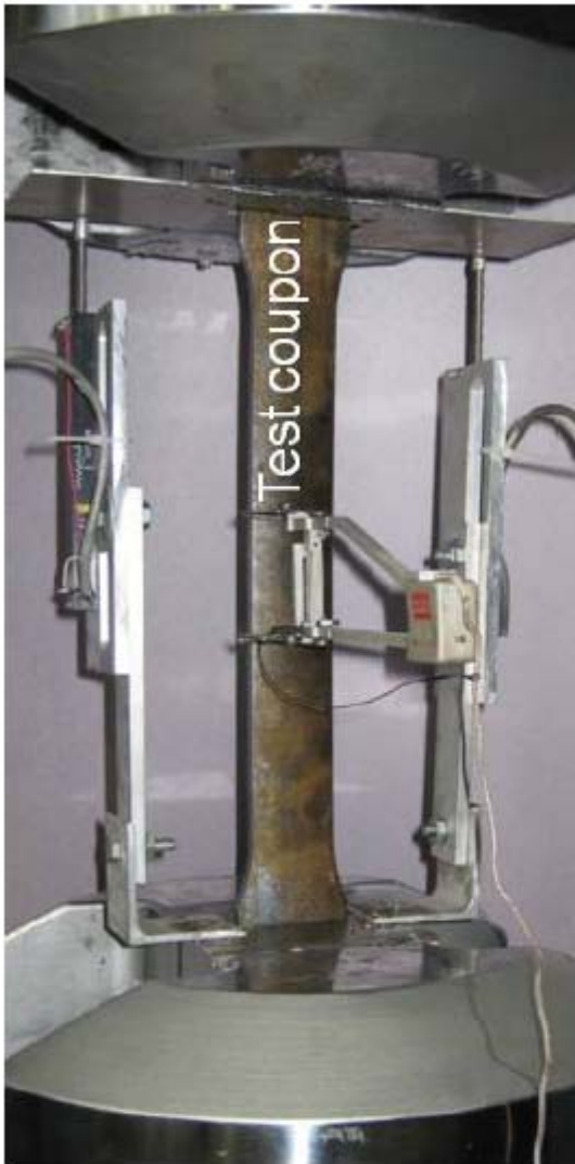
(a) Experimental setup for steel coupon.
