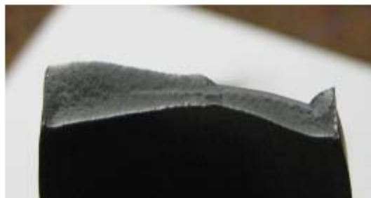
(c) Cross-section of typical fractured test coupon.
