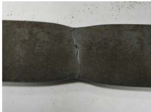
(b) Typical fractured test coupon.
