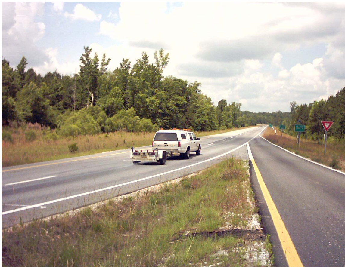
Figure 3.11 Measuring Friction with Skid Trailer.
