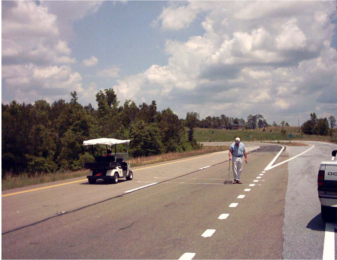
Figure 3.3 Rutting Measurements with Dipstick.
