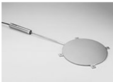
Figure 4.4 Geokon Earth Pressure Cell (Timm et al, 2004).
