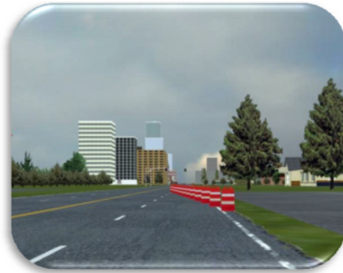
(b) Drums Spaced at 15 ft
