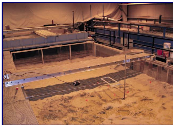
The water/sediment re-circulating flume for the RFID tests (antenna is at the center of the flume)
