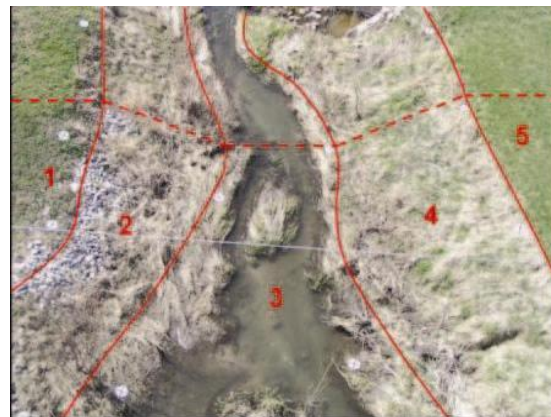
River reach plan decomposition; numbers indicate the quasi-planar surfaces: One and five are floodplains; two and four are sloping banks; three is the river water surface.
