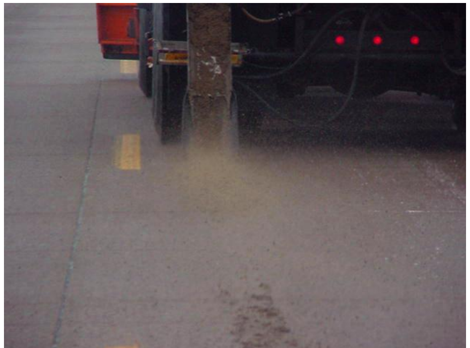
A sander chute in operation mode Photo: The University of Iowa/IHR
