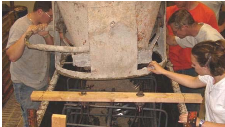
Concrete being placed in the first series of abutment specimen
