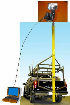
MLSPIV unit with mast deployed and ancillary equipment
