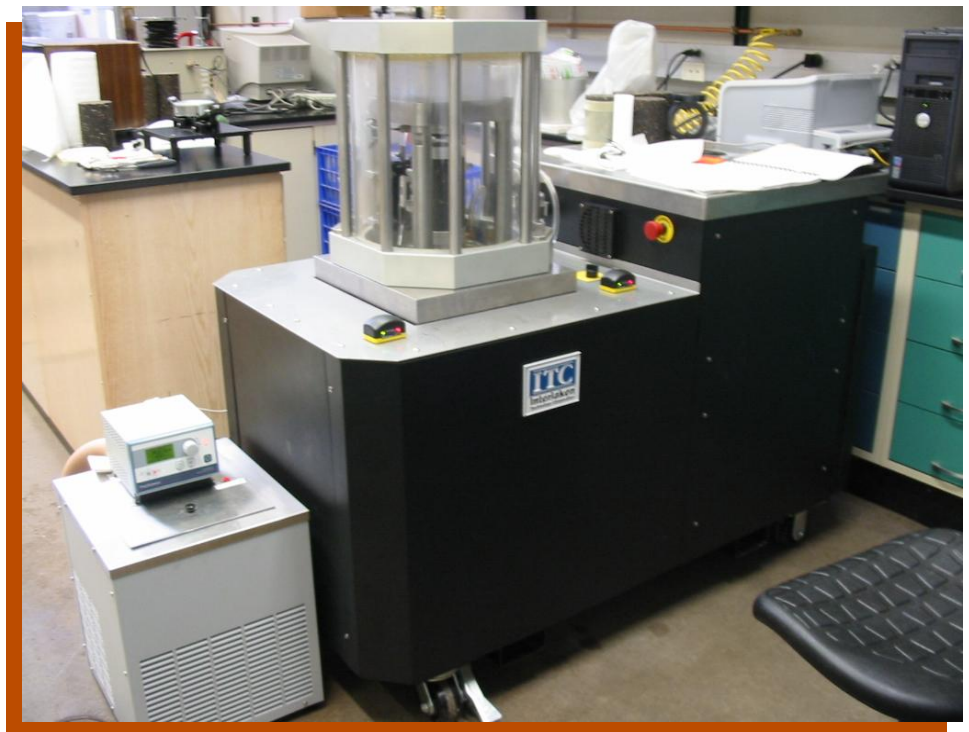
CIR-emulsion mixtures tested using Interlaken Performance Testing Equipment Photo: Dr. Hosin "David" Lee, The University of Iowa/IIHR
