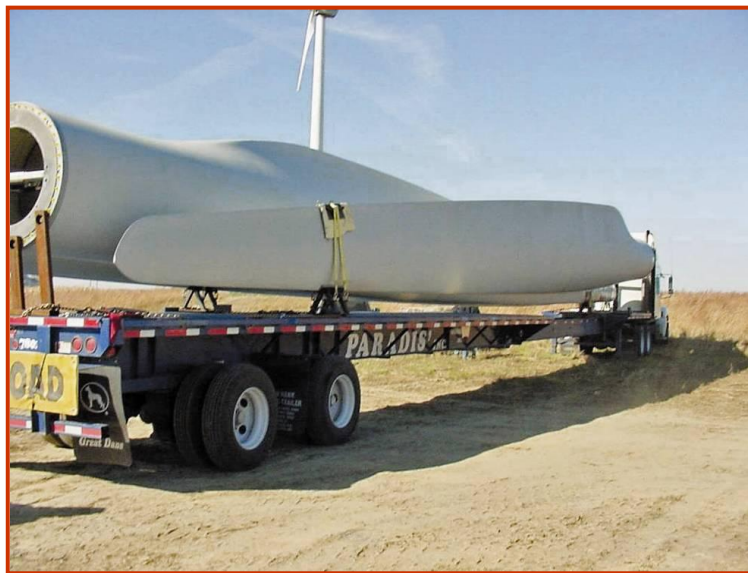
A typical wind turbine blade transport vehicle traveling along Iowa roads. Photo: Iowa Energy Center
