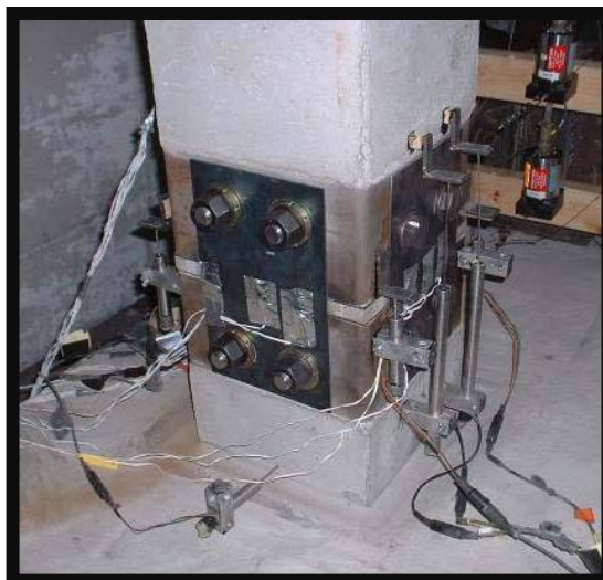
Segmented column joint and foundation prior to testing Photo: Dr. Matt Rouse, Iowa State University/CCEE
