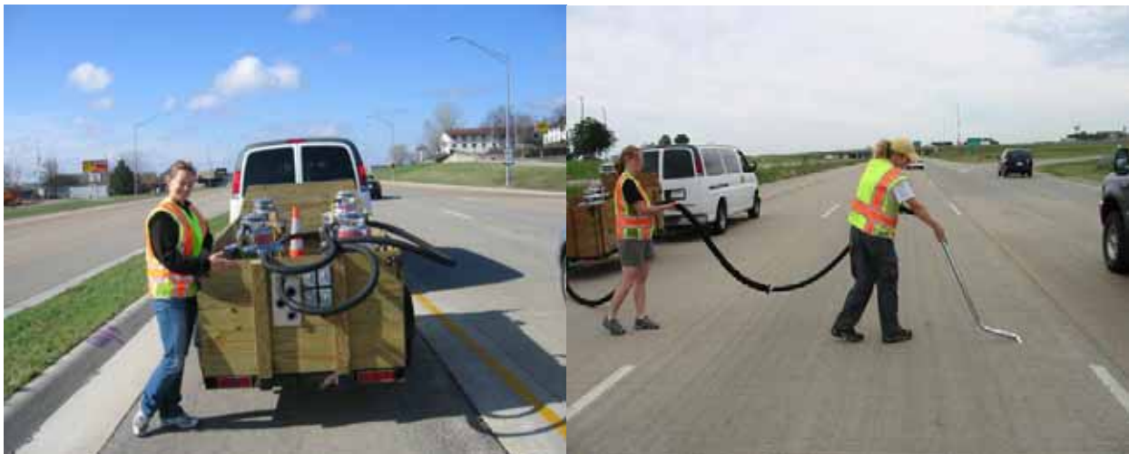
Figure 4. Vacuum trailer set-up; sub-sampling of the freeway.
