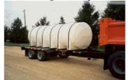
Iowa DOT Trailer 2,700 gallons liquid
