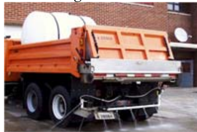
Iowa DOT Combination Unit 900 gallon liquid +6 tons granular
