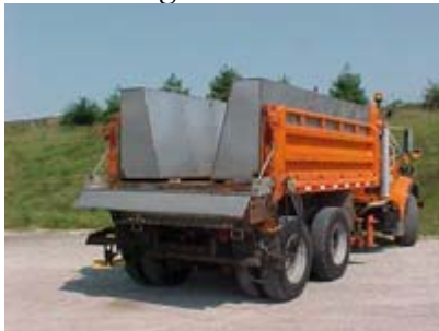
Iowa DOT Combination Unit 1,200 gallon liquid + 5 tons granular
