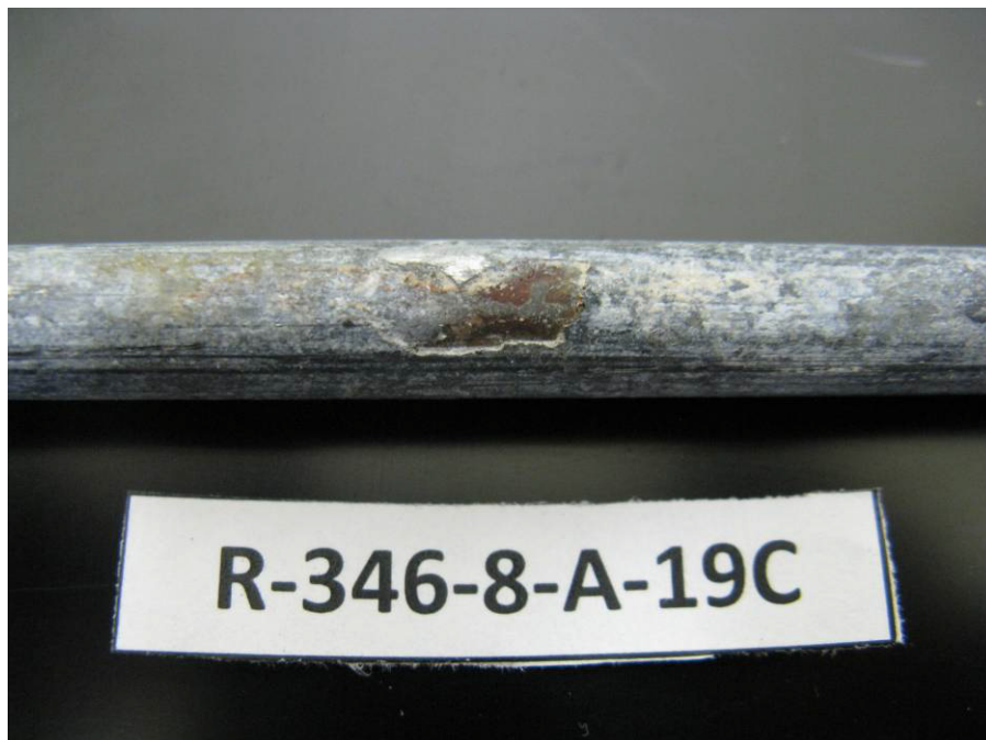
Figure 15 Photograph detailing localized corrosion on coupon R-346-8-A-19, specimen C
