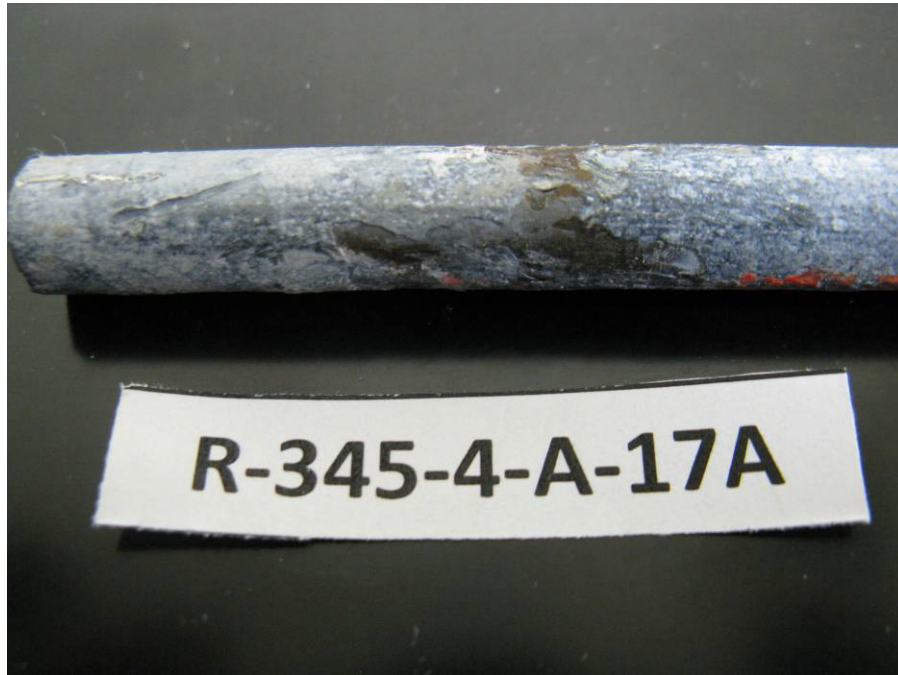
Figure 16 Photograph detailing localized corrosion on coupon R-345-4-A-17, specimen A
