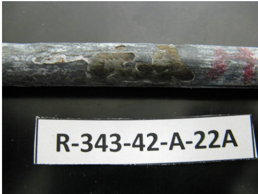
Figure 14 Photograph detailing corrosion of galvanization and steel on coupon R-343-42-A-22, specimen A
