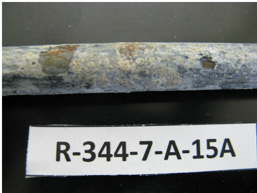
Figure 13 Photograph detailing corrosion on coupon R-344-7-A-15, specimen A
