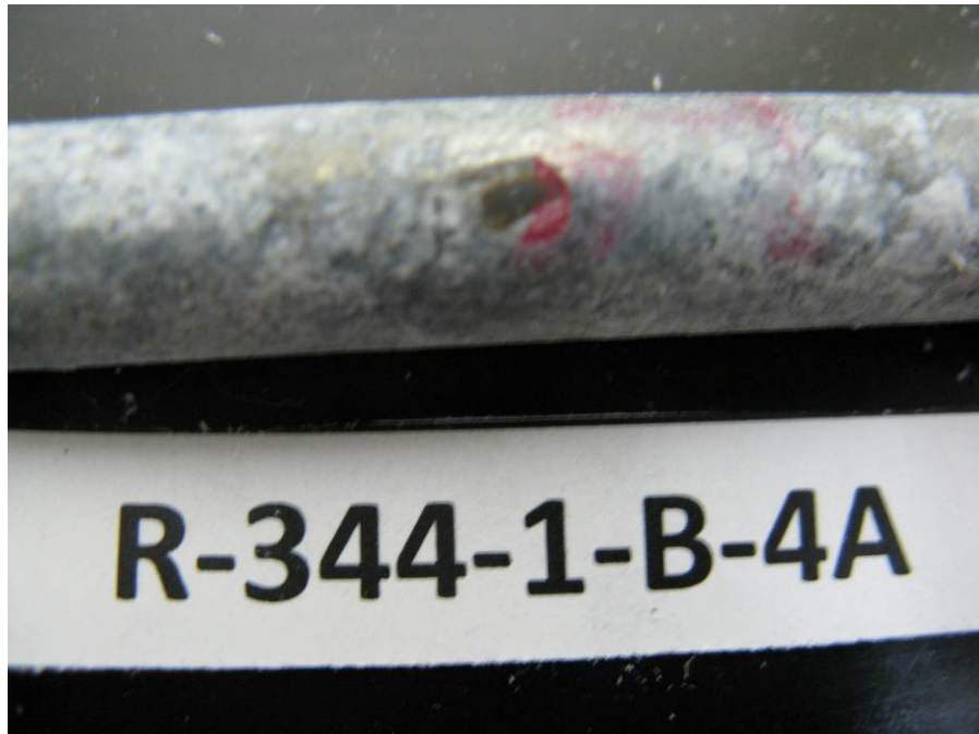
Figure 12 Photograph detailing corrosion by localized pitting on coupon R-344-1-B-4, specimen A
