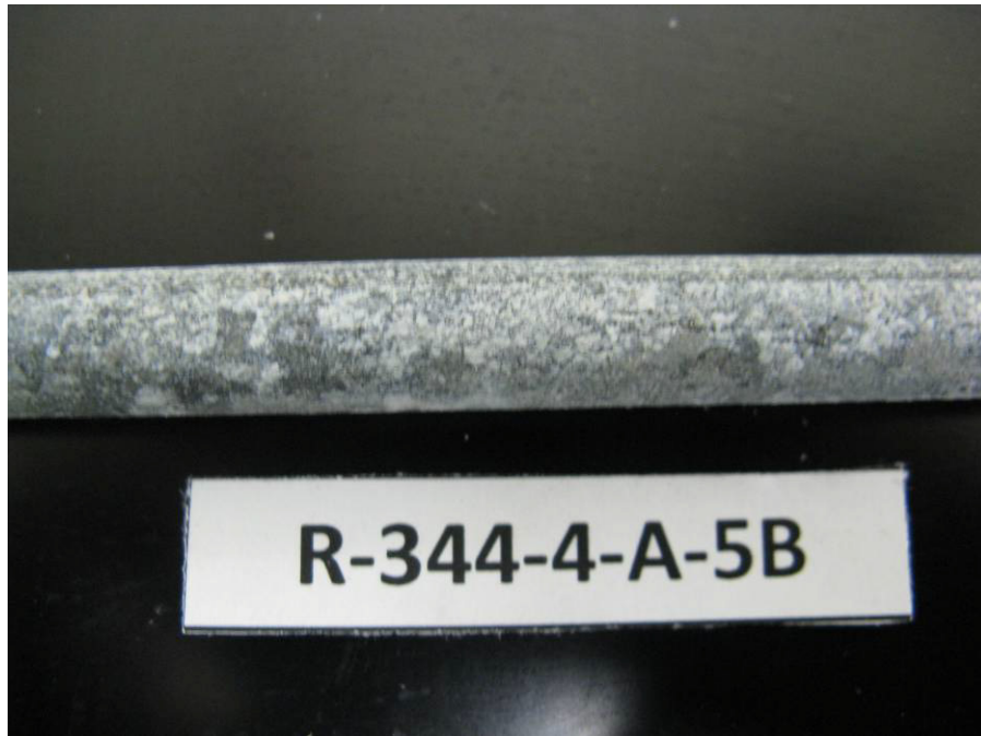
Figure 7 Typical condition of extracted wire coupons
