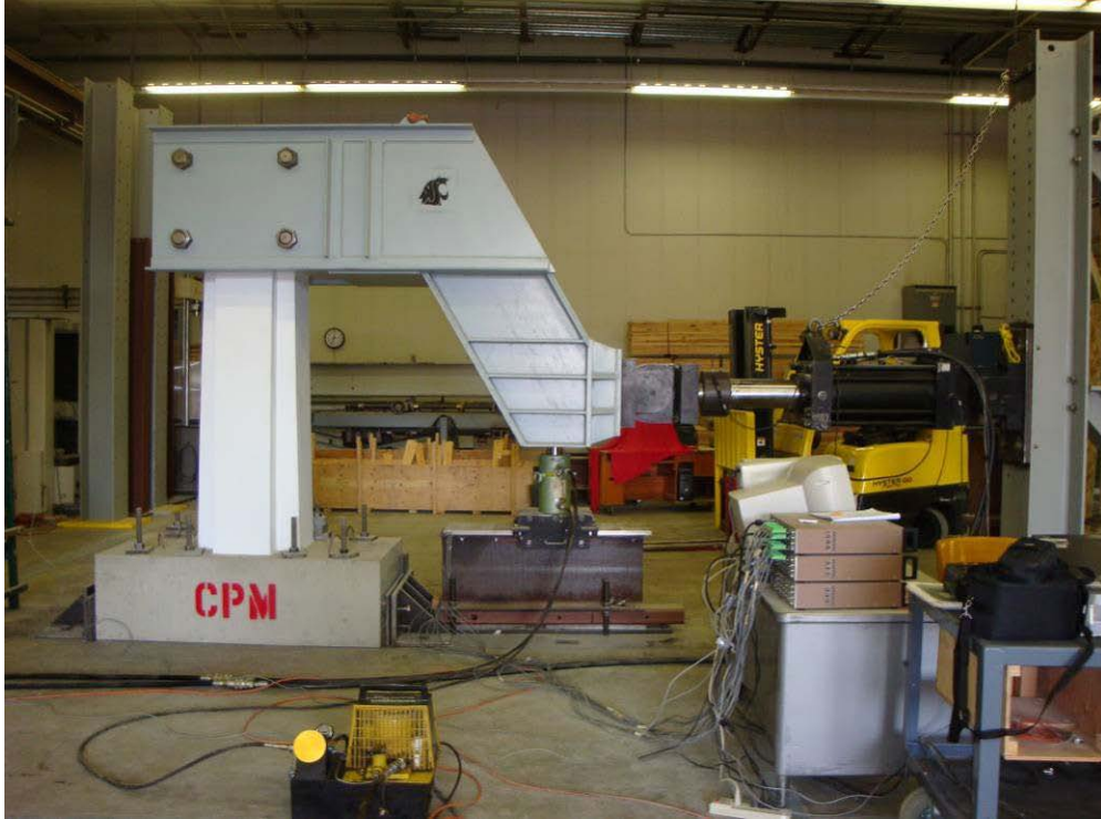
Figure 17 – Column 1 Test Setup
