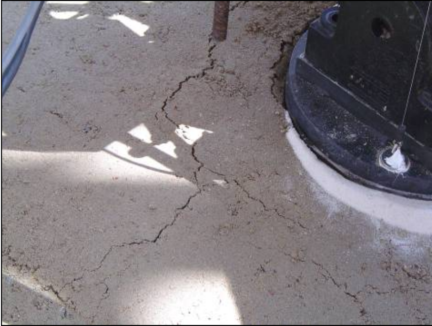
Figure 86. Tension Crack Formation During Cyclic 1 of 17" Select Fill/3" ABC with Geotextile A (8) Test
