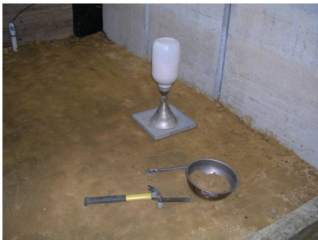
Figure 62. Typical Sand Cone Test Setup
