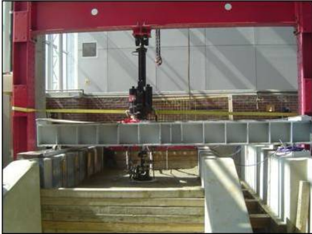
Figure 49. Completed Test Section Showing Test Pit, Load Actuator, and Reaction Frame
