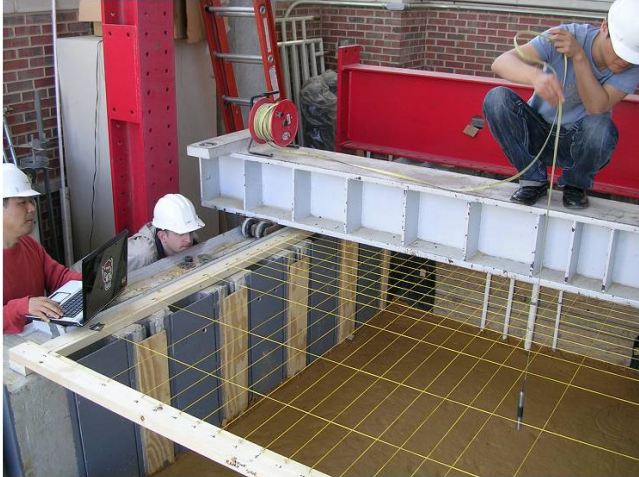
Figure 53. Typical surface profile measurement
