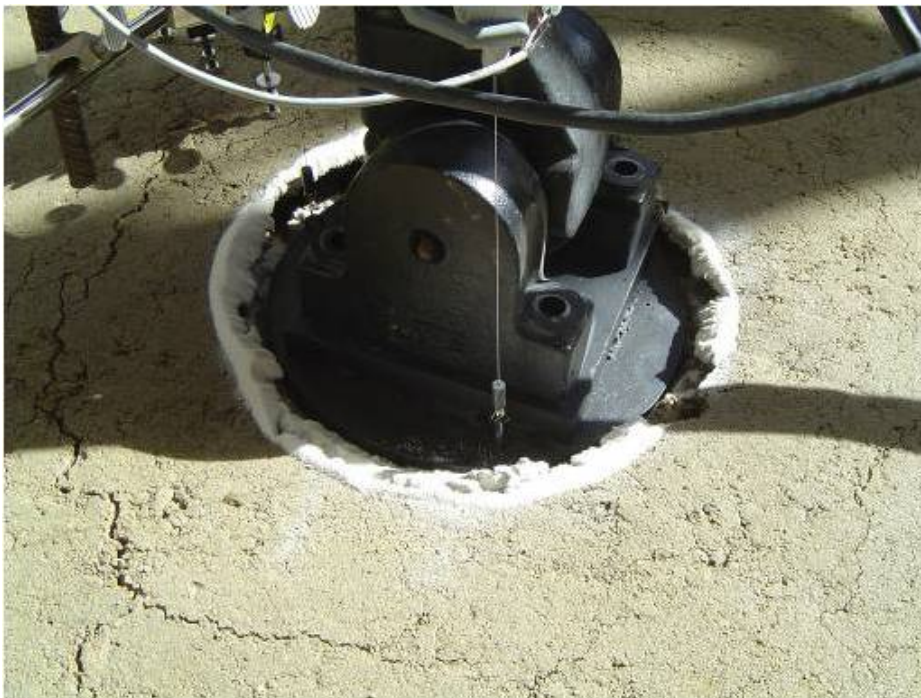
Figure 90. Punching Failure during 14" Select Fill/3" ABC with Geotextile A (11) Test
