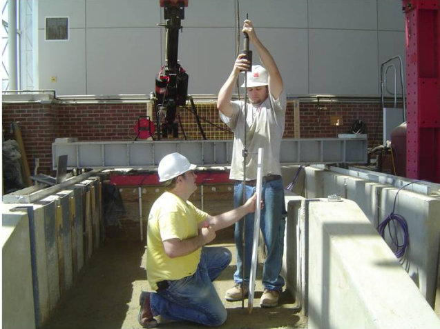
Figure 64. Typical Dynamic Cone Penetrometer (DCP) Test
