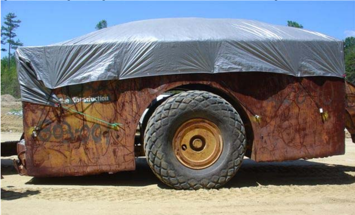
Figure 35. Proofroll trailer (courtesy M. Valiquette, NCDOT)
