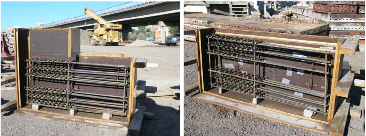
Figure 3: Forms for Pullout Specimens
