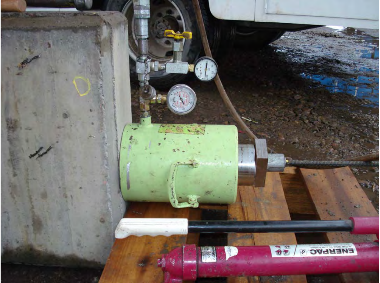
Figure 4: Pullout Test Apparatus
