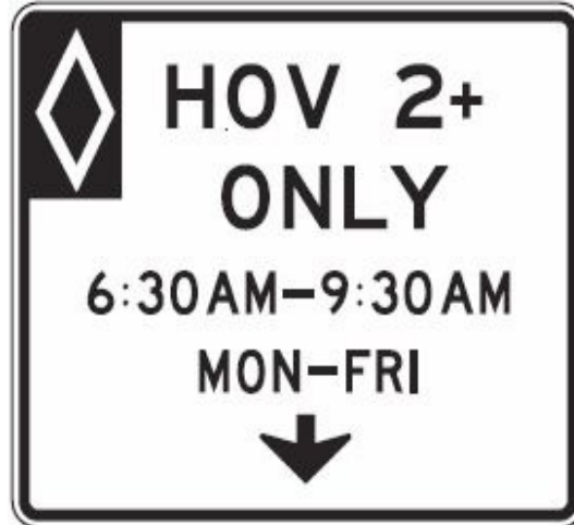
Figure 2-15. Overhead HOV lane sign (FHWA 2003)
