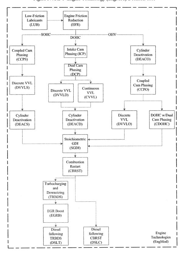
Figure IV.C.2-1 Engine Technology (EngMod) Decision Tree
