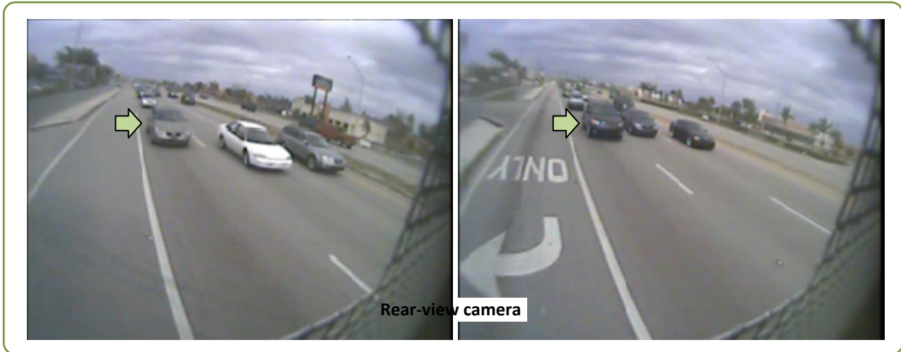
Figure 15: Screenshot of vehicle yielding to bus on test corridor in Fort Myers.
