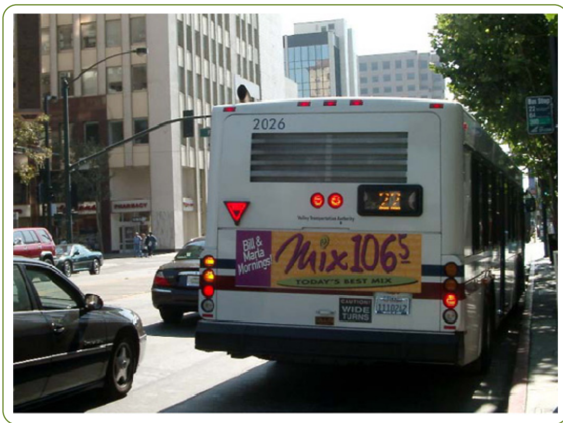
Figure 30: Yield LED sign on VTA buses.
