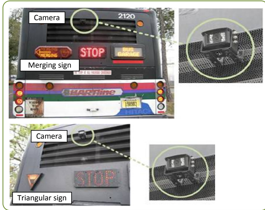
Figure 9: Sign installation and data collection setting for HART.
