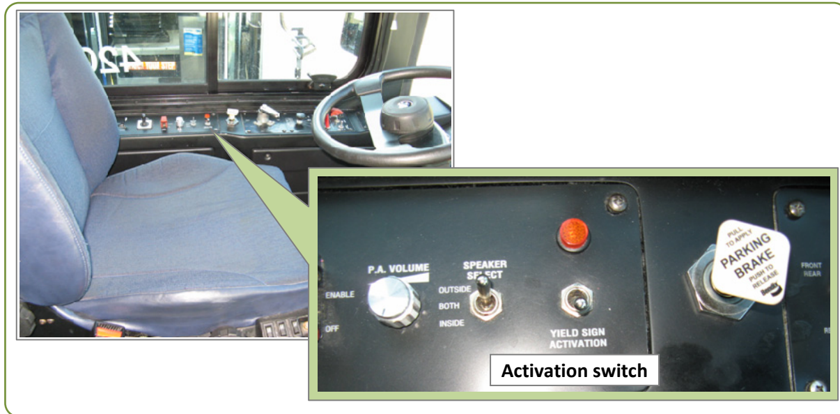
Figure 7: YTB-LED sign activation switch.
