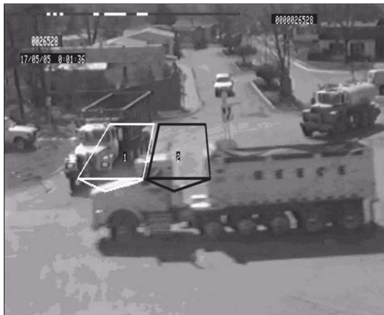
Figure 21. Example Using Traficon Directional Detectors.
