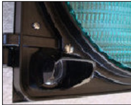
Figure 25. Close-Up of ITS Plus Camera Mounted in Signal Head.
