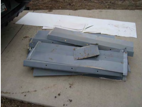
Figure 17. Bird Slide panels and white plastic panels collected after December 2008 wind storm.
