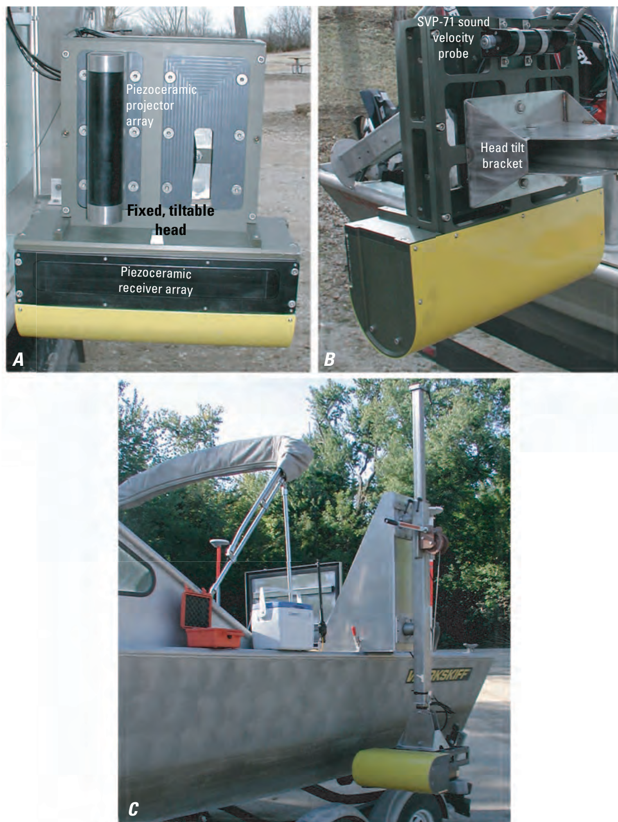
Figure 2. The multibeam echo sounder as viewed A , from the bottom, B , from the top, and C , mounted on the port side of the U.S. Geological Survey boat.
