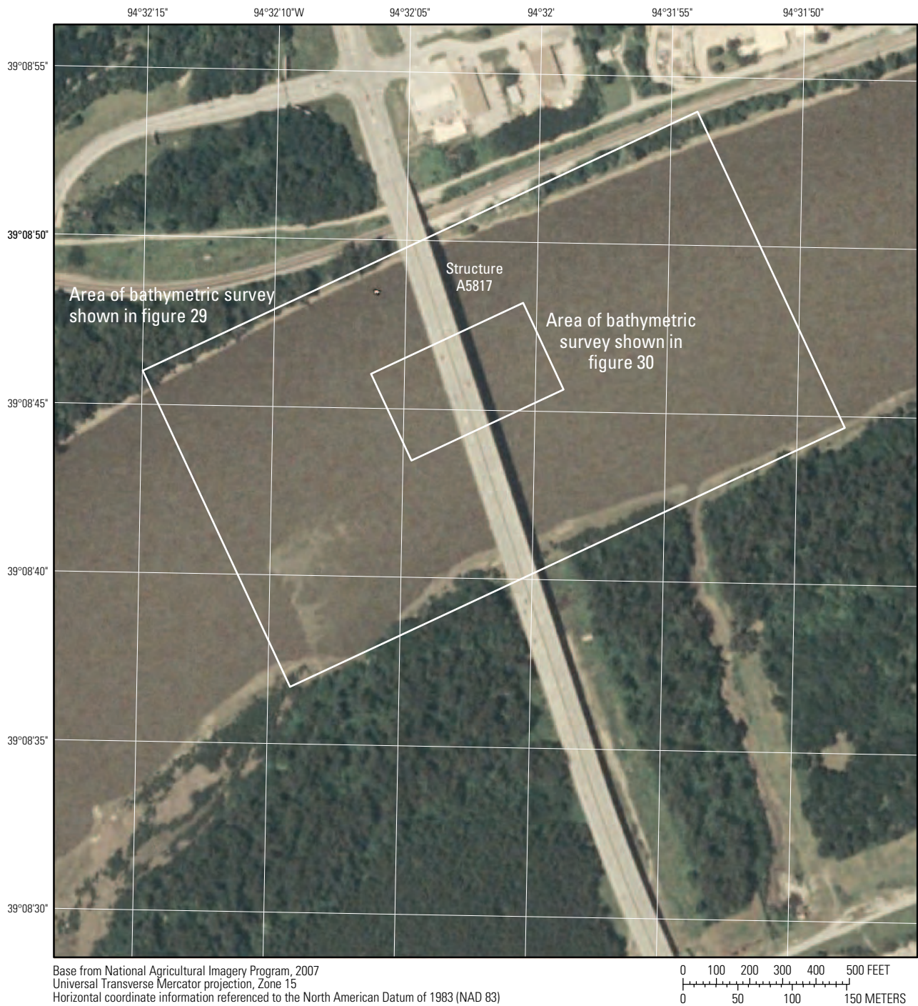
Figure 28. Location of the bathymetric survey area on the Missouri River near structure A5817 on State Highway 269 in Kansas City, Missouri.
